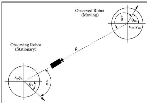
Figure 2: Observation of the Moving Robot by the Stationary Robot. Note that the “camera” indicates the robot with the Robot Tracker
