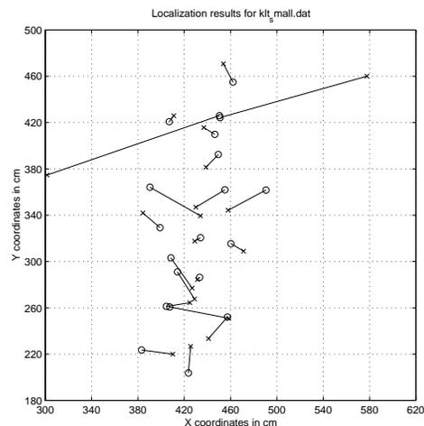
Figure 9: Tracker estimates vs Image-based estimates for a set of 21 random positions.
