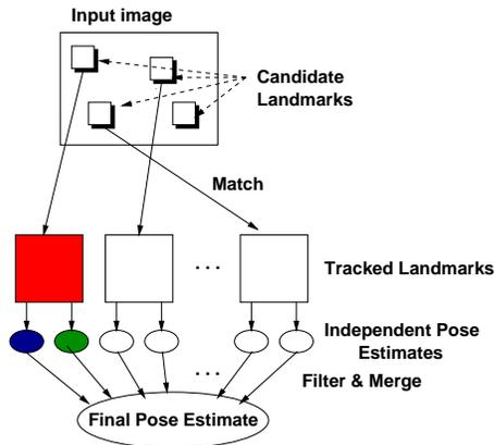
Figure 4: Pose estimation based on learned visual landmarks. Landmarks (small squares) are extracted from the current camera observation and matched to the previously learned tracked landmarks. Each match generates a pose estimate, which are filtered and combined to generate a final pose estimate.
