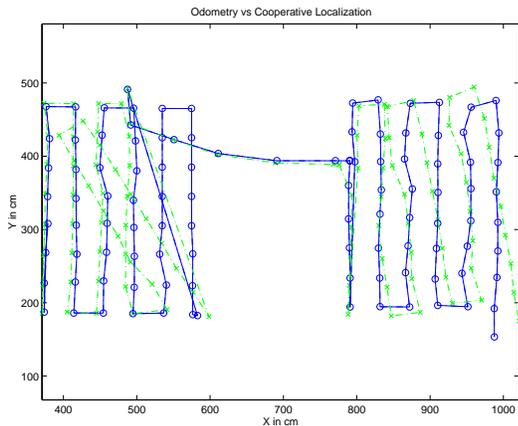
Figure 6: Odometric (x) vs Tracker-corrected (o) trajectories of the robot.
