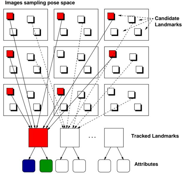
Figure 3: The off-line training method. Images (large rectangles) are collected sampling the pose space. Landmarks are extracted from the images and matched across the samples. The tracked landmarks are parameterized as a function of pose and saved for future pose estimation.
