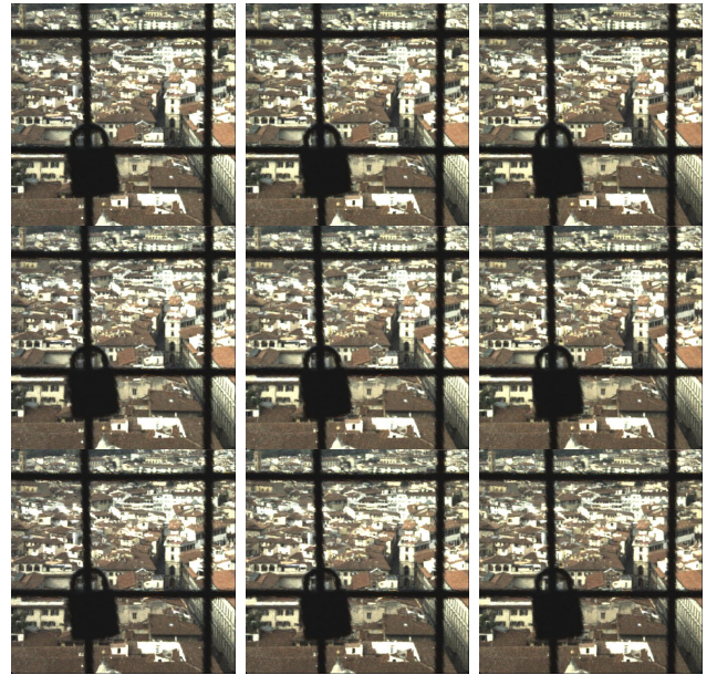
Fig. 2. The central 9 sub-aperture images of our illustrative example. While they appear quite similar, the foreground region (the black pixels) shift by about 7 pixels between neighboring images. Note: these images look low quality because they are from raw sensor values; they have not been transformed to SRGB space, tone-mapped by the camera response function, or white balanced.
