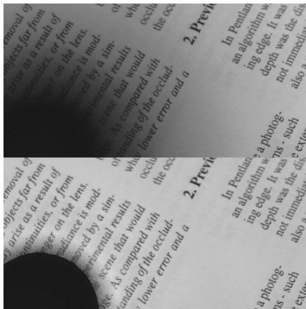
Figure 4. Camera (top) and processed (bottom) images with an occluding object.
