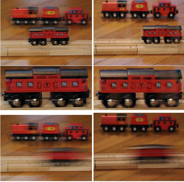
Figure 7. Comparing the performance of a half parabola (left column) with the full parabolic motion invariance (right column). When the motion prior is asymmetric, and a half parabola is used to capture rightward motion, the reconstruction has higher contrast and less noise. The first row shows a scene with rightward motion, and the second row shows a closeup of the train. Reconstruction quality is higher from the half parabola, though both images have reconstruction artifacts due to specular reflections off of the metal parts of the wheel. When the motion does not obey the asymmetric prior distribution, the half parabola cannot give a good reconstruction (third row, left); a traditional image capture with the same object velocity and exposure time is shown (third row, right).
