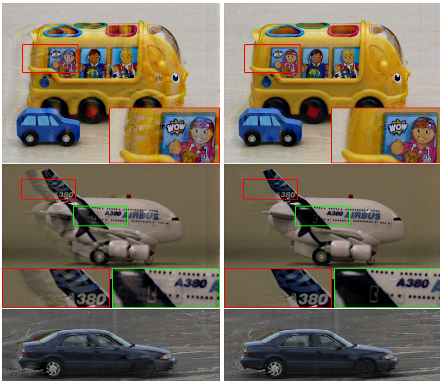
Fig. 8. Experimental results with our real camera. Left column shows the result of deconvolving B_0 , as in previous motion invariant work. Right column shows the result of deconvolving B_s , after applying our motion estimation algorithm. Echo artifacts are noticeably reduced when deconvolving B_s . Best viewed electronically.
