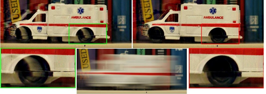
Fig. 1. (Top left) A motion invariant image, deblurred as in previous work. The invariance approximation results in artifacts, most notable in the wheel area. (Top right) Using our motion estimation algorithm, we avoid these artifacts and improve the quality of the reconstruction. (Bottom row) zoomed views of annotated regions, plus a traditional image of the moving object to convey the extent of motion.
