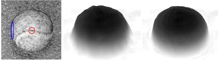
Fig. 5. (Left) Image of a tennis ball on a ground plane annotated with measurement regions. (Center) Surface plot of depth measured over circular regions. (Right) Surface plot of depth measured over ellipses evolved to approximate equifocal regions.
