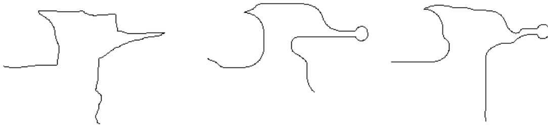
FIGURE 6.7. Results with and without the magnetic regularization term. The left path shows the goal trajectory, the middle shows the resulting output without the magnetic regularization term and the right path shows the output with the magnetic regularization term. The cusps indicate a direction reversal.
