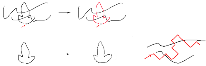
(a) Example extraction and refinement. Top left shows original image and the user pointer, top right shows the automatically selected curve (in red). Bottom left shows the curve isolated by dragging it and bottom right shows result of the automated refinement process.
