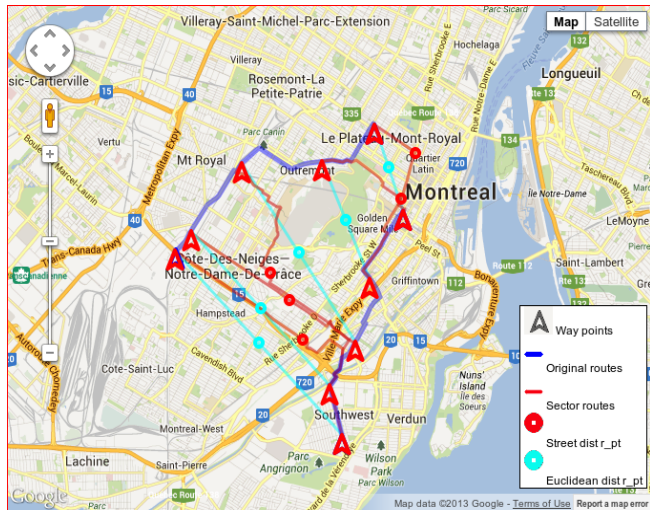
Fig. 1: An instance of rendezvous planner using Google maps API ©. The blue solid lines on the map indicates individual agent trajectories, red arrows indicate waypoints, cyan circles indicate rendezvous points computed using Euclidean metric and red circles indicate rendezvous points generated using actual travel times on the road network.
