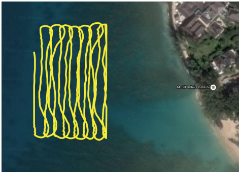
Figure 6: Sparse lawnmower trajectory performed by the boat to collect the bathymetric data to create the depth map.
