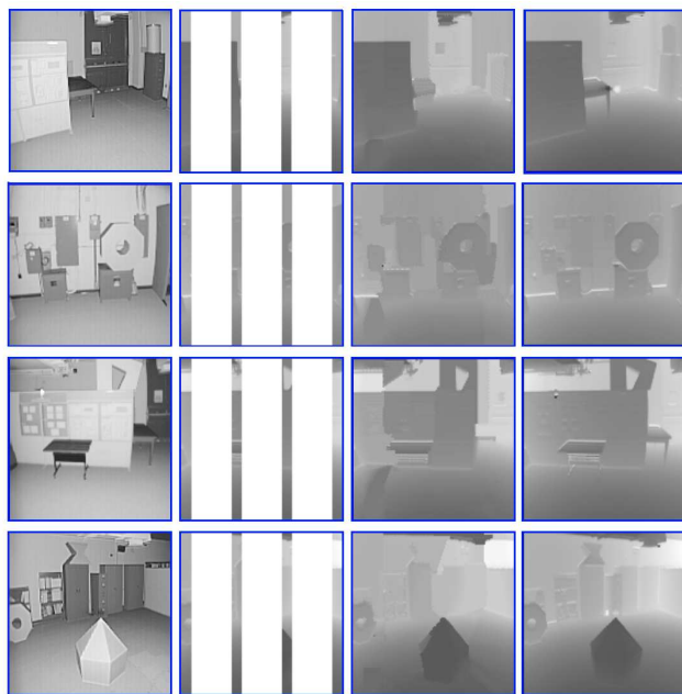
Figure 10: Examples on real data for the case of subsampling with r_w = 8 and x_w = 32 . The first two columns show the input intensity and range data, respectively. The last two columns show the synthesized results and the real range images for visual comparison.
