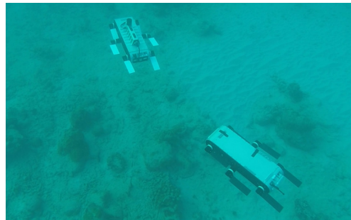
Fig. 6. Pair of Aqua robots following one another at sea and positioned for gesture-based communication.
