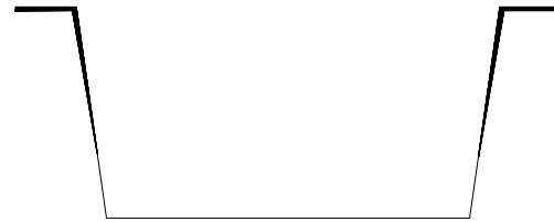
Figure 2.2b: material distribution for female molded part
