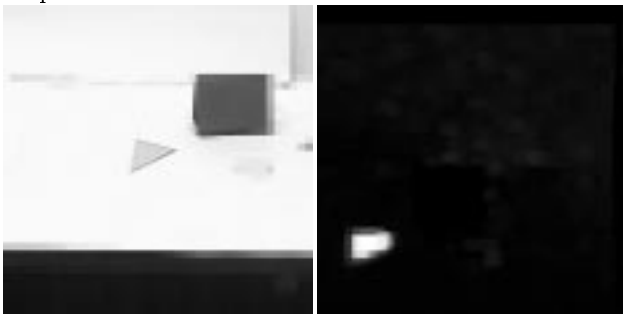
Figure 2: Left: The foveal image of the scene, just after a camera movement based on a target colour of red. Right: The corresponding head centred saliency map.
