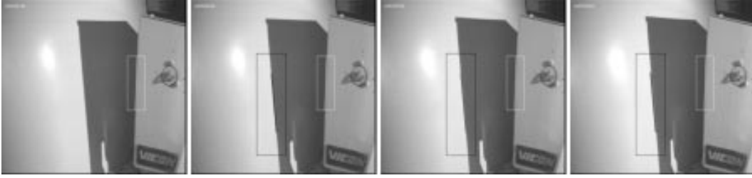
Figure 3: A series of images captured as the light source moves. The white and black rectangular outlines are overlaid by hand and serve as constraint regions for the shadow boundary detection algorithm. Enclosed in the white box is the self cast shadow, i.e., the portion of the object edge of interest. Enclosed in the dark box is the region in which we wish to find the corresponding cast shadow.
