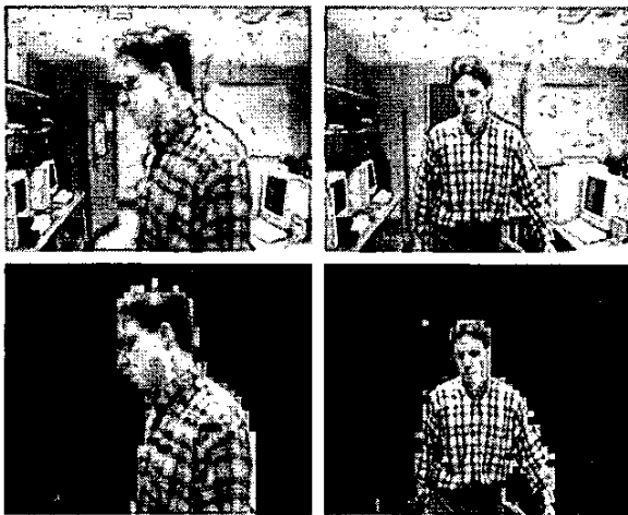
Figure 2. Snapshots of the background modelling process run on a scene containing an opening and closing door. All images come from a single sequence.
