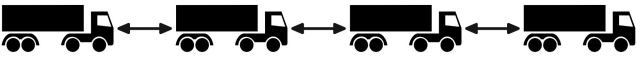
Fig. 4. A four agent vehicular platoon. The arrows indicate communication links between the agents.
