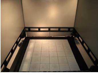
Figure 1: Left: The floor interface is situated within an immersive, rear projected virtual environment simulator. Middle: Sensing and actuating components are integrated beneath the floor. Right: View from above showing sensor locations.
