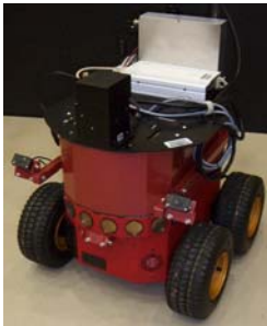
Figure 11 - The Mobile Robotics Test-bed
