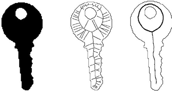
Figure 4. The image of a key (left) and its (endo-) skeleton corresponding to different levels of significance (middle and right).
