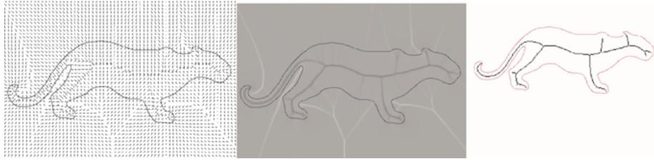
Figure 6. The gradient vector field of the Euclidean distance function of the boundary of an object (left), the average outward flux (middle) computed over a  $3 \times 3$  circular neighborhood, and the computed skeleton (right) obtained by homotopy preserving thinning (see Section 5.2).
