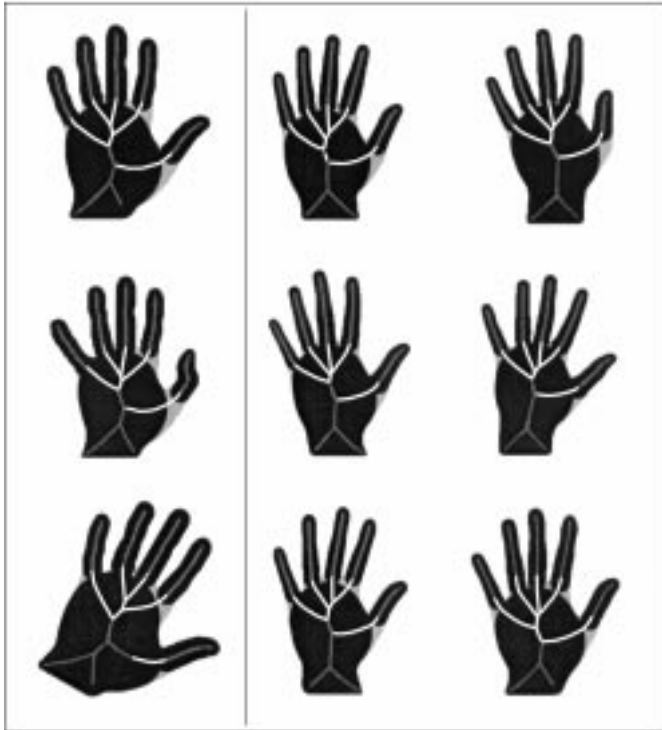
FIG. 10. (Top) Grey-scale image obtained for topological sensitivity experiment (see text). (Bottom box) Similar shapes with distinct internal skeleton topologies (compare left to right two columns). Grey lines represent combined bends/seeds and nonligature. Note how ligature (white) highlights the topologically distinct skeleton regions, making explicit (in the remaining skeleton) the perceptual similarity of all these objects.
