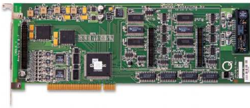
Figure 5: Q8 hardware-in-the-loop (HIL) PCI control board
