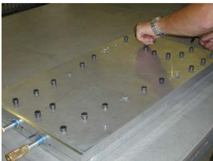
The cap screws must be loosened at about the same rate. Otherwise much greater torque is needed to unscrew the mold.
