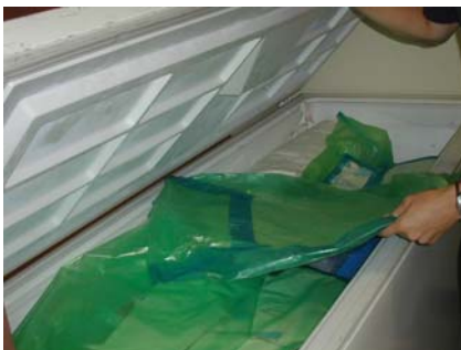
Each of the pieces of pre-preg material should be kept in the freezer until the time when they must be placed into the mold. Otherwise the material becomes very tacky and hard to maneuver.
