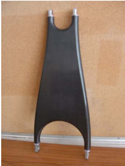
Figure 78: The carbon fibre actuator arm is complete.
