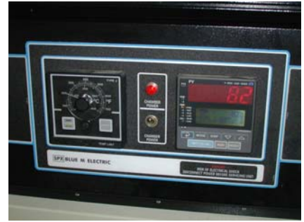
The oven control panel stores the program, after which a simple 'Start' is needed to begin.
