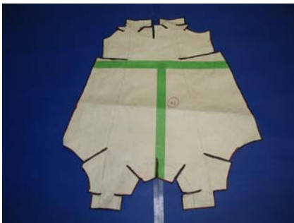
Pieces 2 & 3 - (Qty: 1 & 1) Interior layer meant to have flaps that can be overlapped. Piece 3 is the mirror or Piece 2.
