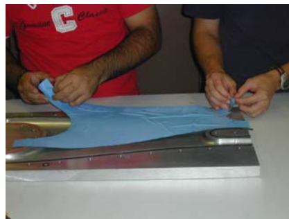
Piece 1 is the first to be placed. One piece must be placed carefully on the top of the mold, and similarly another on the bottom of the mold.
