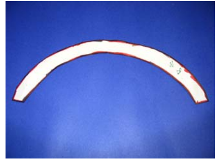
Piece 1-B - (Qty: 2) Patch for openings created by cuts in Piece 1 on wide end.
