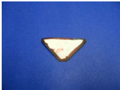
Piece 2-A - (Qty: 4) "Triangle Patch" used to cover large opening created by cuts in Pieces 2 & 3.
