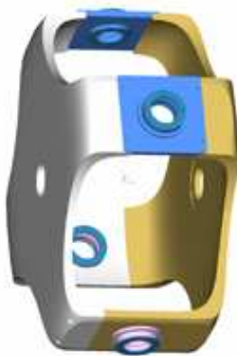
Figure 7: The Stephenson-linkage housing made up of two identical covers
