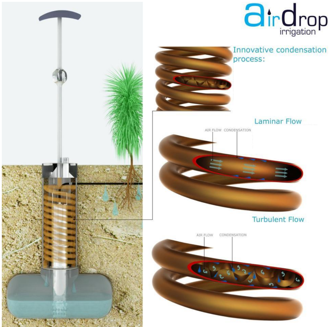
Figure 6. Innovative condensation process
