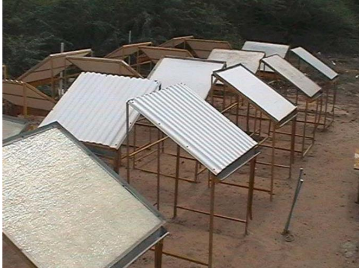
Figure 12. Different Condenser Surfaces Sample Tests
