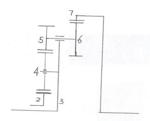
When Gear 7 is fixed, W7=0. and Wz=-100rev/min. CW.
