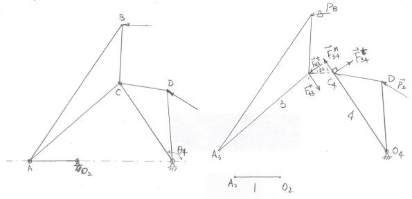
Decompose the system into parts, and first consider Body 4,
