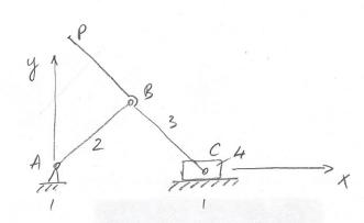
$$R_{SA} = R_{CB} = R_{PB} = 25 mm$$
