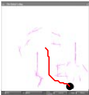
Fig. 15. Dynamic Mapping and Trajectory Determination. As the robot moves towards a pre-defined spatial location, sonar data update the map and alter the trajectory.
