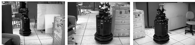
Fig. 16. Autonomous Navigation with No A Priori Map. The robot successfully navigated around various obstacles as it traversed towards a pre-defined spatial location.
