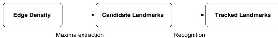
Fig. 3. The training process: Candidate landmarks are detected as local maxima of edge density and then tracked into sets of tracked landmarks.
