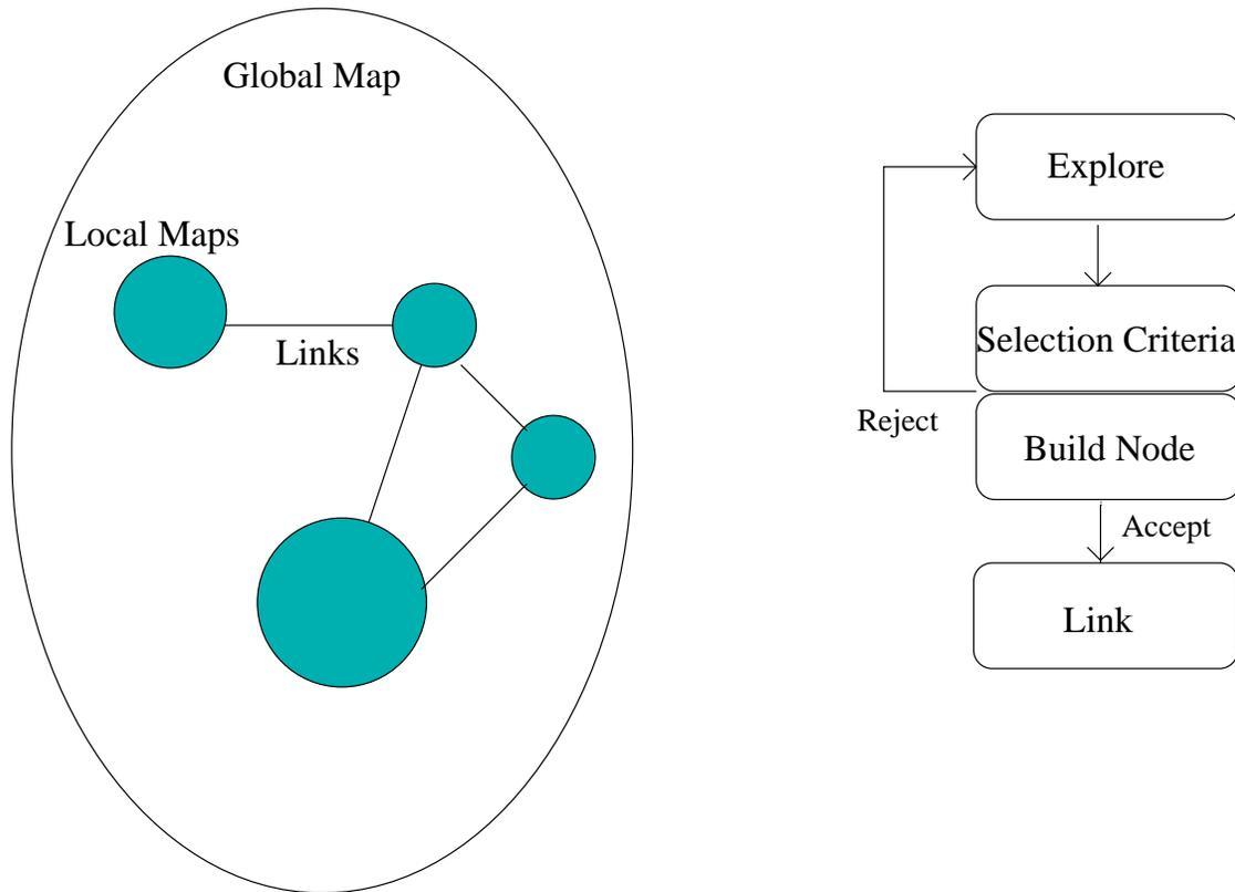
FIGURE 1. A global map composed of connected local maps (left) and a flow chart of the map construction algorithm (right). The robot explores until the selection criteria are activated. At that point, the robot builds a local map while intermittently confirming that the criteria evaluation is still positive. Once the local map is complete, it is linked to the hierarchy of local maps previously constructed.
