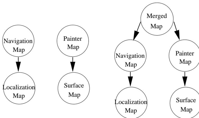
FIGURE 1. An example of 2 task-based maps. A navigation map consisting of connected localization maps and a painter map consisting of connected surface maps (describing the surfaces to be painted). The merged map allows the robot to navigate and paint the environment.
