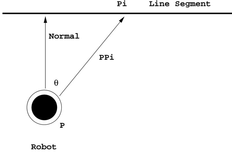
FIGURE 1. Sweep over each line segment to determine the overall constraint and reliability. Scanning resolution can be continuous or match that of the real sensors.
