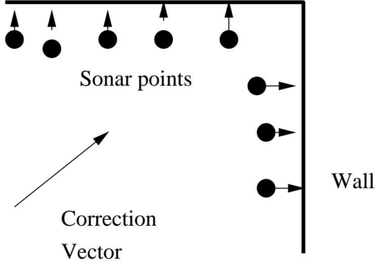
FIGURE 2. Localization by iterating about the Correction Vector consisting of a weighted sum of the error vectors.
