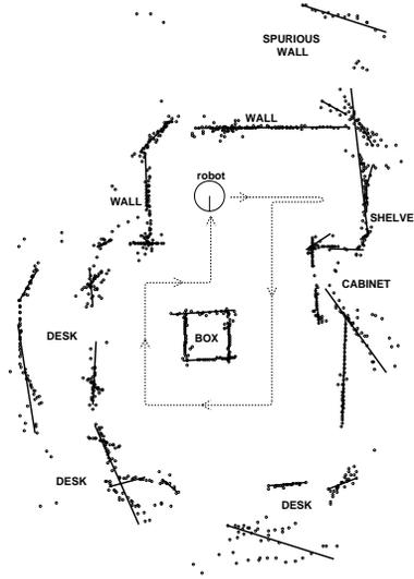
FIGURE 1. An environment modelled by line segment fits [1]. A robot explored the environment, following the dotted path, to build the line segment model.
