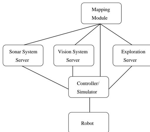
FIGURE 1. Flow chart of software modules.
