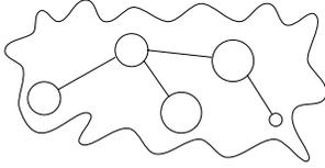
Fig. 1. Global map composed of a set of local maps. Circles represent metrically accurate local maps.
