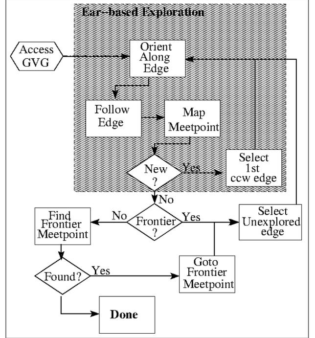
Figure 3. Ear-based exploration using the GVG representation.
