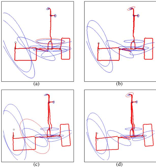
Figure 7. (a) shows the map  $2\text{-}\sigma$  uncertainty ellipses after exploring the entire environment without re-localizing during exploration (b) shows the map uncertainty reduction after performing re-localization (c) and (d) show the same maps as in (a) and (b), except that re-localization was performed during exploration of the environment (prior to the map shown in (c)).
