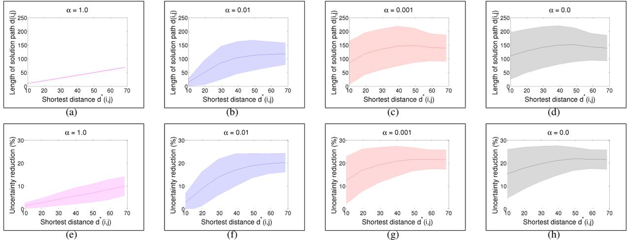
Figure 5. (a)-(d) Error bar plots showing length of the solution path  $d^*(i,j)$  compared to the shortest path distance using  $\alpha = 1.0, 0.01, 0.001$  and  $1.0$  for (a) through (d), respectively. (e)-(h) error bar plots showing total uncertainty reduction (in %) from single re-localization for all pairs  $(i,j)$  again using  $\alpha = 1.0, 0.01, 0.001$  and  $1.0$  for (e) through (h), respectively.
