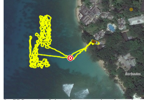
Figure 8: GPS track of the robot executing the trajectory from selective coverage. The figure also shows the deployment phase on the shore.
