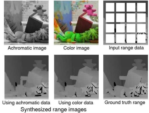
**Figure 2. Results on achromatic and color images. The MAR error is 7.71 when using grayscale and 6.39 when using color information.**
