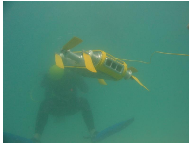
Fig. 4. Visual servoing off a yellow target, open ocean trials.
