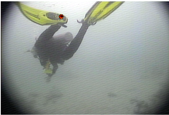
Fig. 3. Flipper tracker tracking diver's flippers: Sequence 1. The circular mark on the heel of the left flipper is the target location determined by the system.
