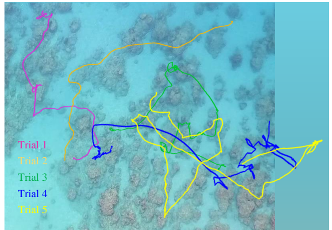
Fig. 7. Planar projections of estimated paths executed during five trials of our experiments (each in a different color). An aerial view of the reef is used as a background to show underlying coral structures and was not available in acceptable quality for the right edge of the region being displayed.
