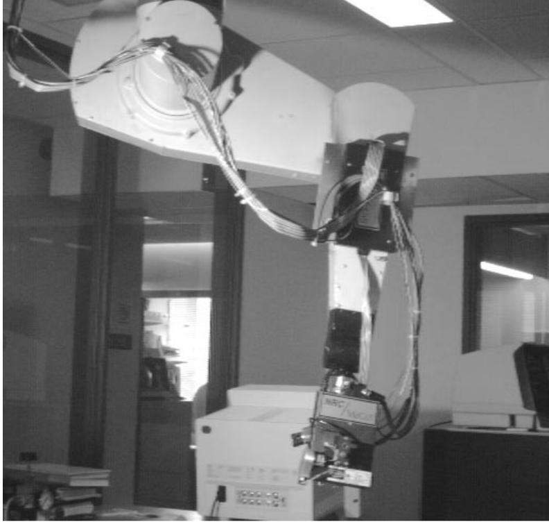
FIGURE 2. Mobile scanner setup. A laser rangefinder with a  $1m^3$  field of view is mounted on the end-effector of an inverted Puma 560 robot.
