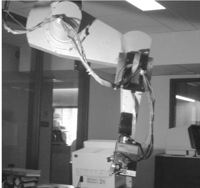
FIGURE 13. The mobile sensor consists of a laser range-finding system with a  $1m^3$  field of view mounted on the end-effector of an inverted PUMA 560 robot.
