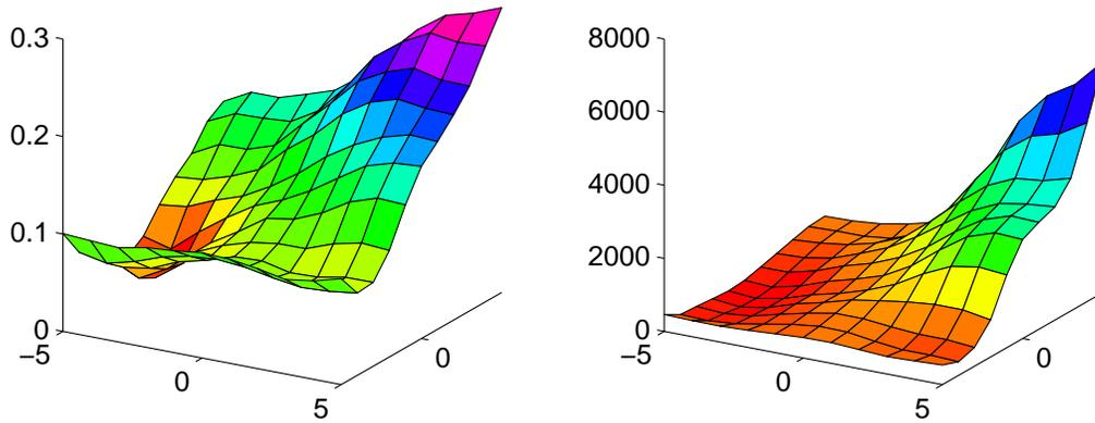
FIGURE 3. **Region Matching Zone 1.** The error surfaces generated using the normalized error measure versus the SSD error measure. The vertical axis is the error, the x and y axes are the pixel region shifting between the two frames to obtain the region match. This corresponds to a corner of the cube in the image sequence. Note the minima in the lower left of the two surfaces, where the true correspondence lies.
