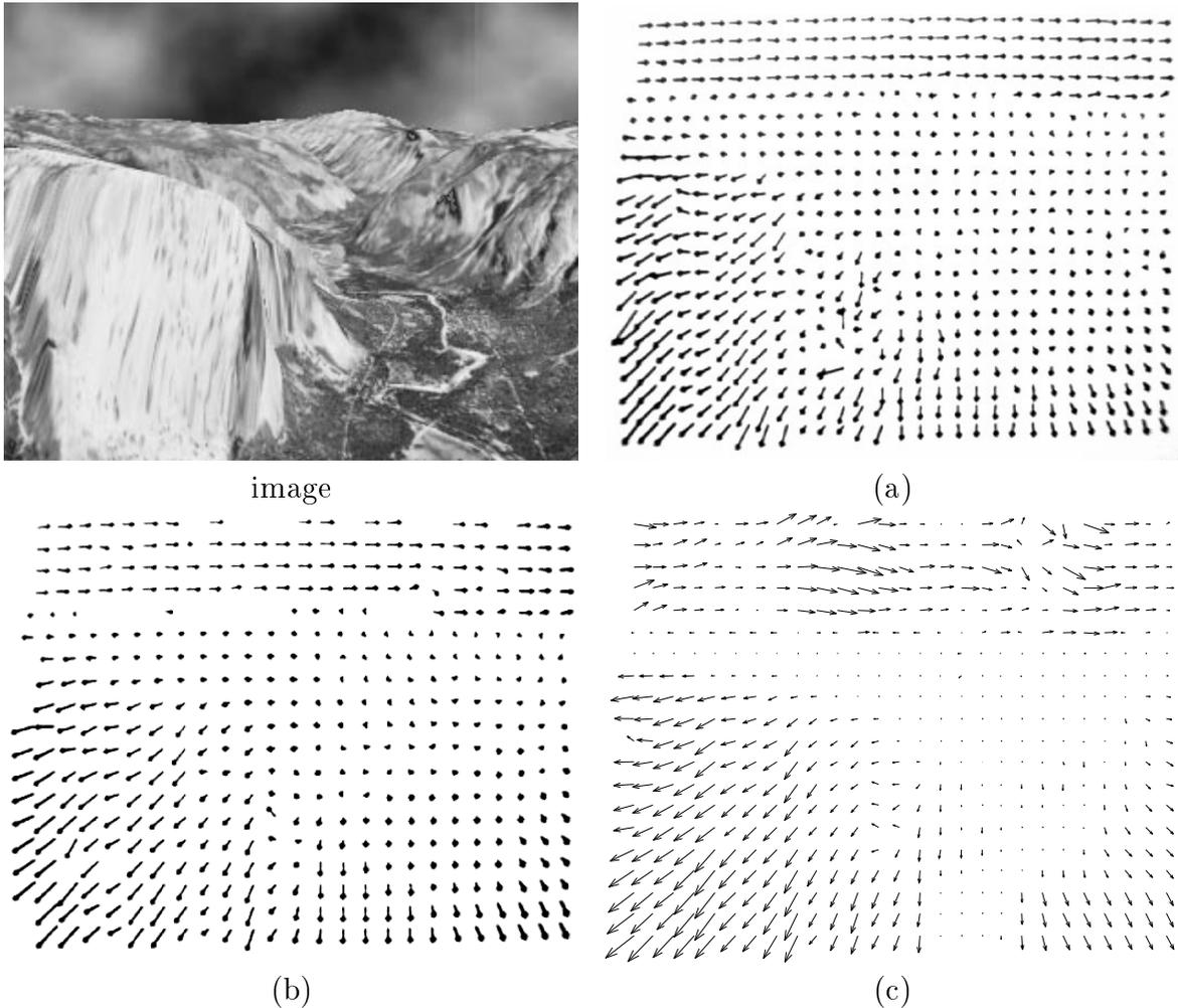
FIGURE 5. **Yosemite Sequence, Performance Comparison.** The flow field for Anandan’s algorithm is shown in (a). Singh’s algorithm produced the flow field shown in (b). Both plots were obtained from [4]. Our results were resampled and are shown in a similar format in (c).
