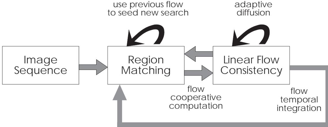
FIGURE 1. Block diagram of full optical flow process.
