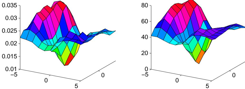
FIGURE 4. **Region Matching Zone 5.** The error surfaces generated using the normalized error measure versus the SSD error measure. The vertical axis is the error, the x and y axes are the pixel region shifting between the two frames to obtain the region match. This corresponds to the poorly-lit, our-of-focus whiteboard in the background in the image sequence. Note the SSD error surface does not tell us how ambiguous the overall matching is.
