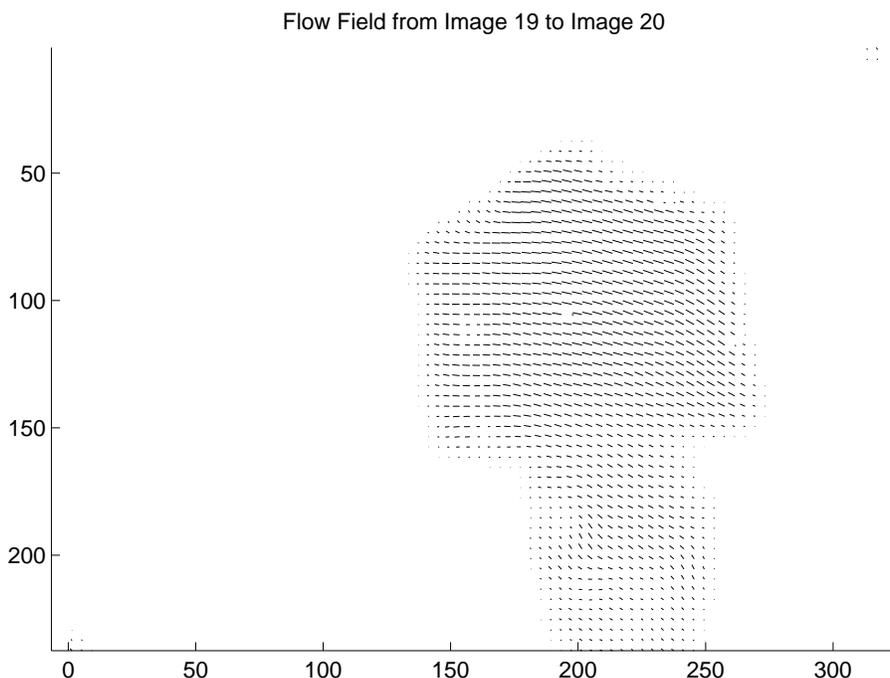
FIGURE 11. **Hand-Held Target Sequence, Flow Field.** The measured flow field between frames 19 and 20.
