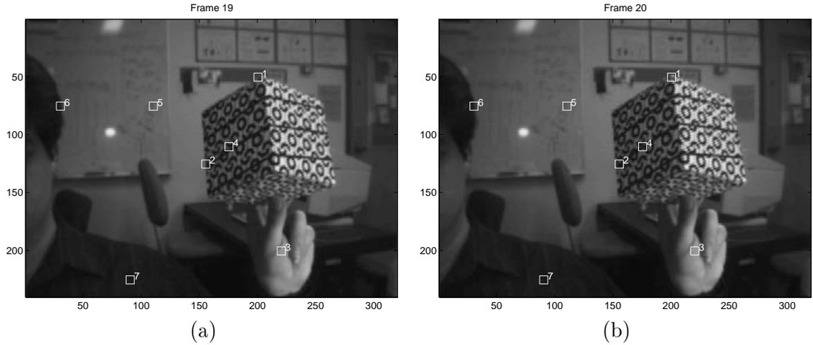
FIGURE 2. **Region Matching image frames.** Frame 19 of the hand-held moving cube (a), and Frame 20 (b). The numbered squares are the initial tile positions for region matching between the two images. The number corresponds to the region matching experiments, shown later.
