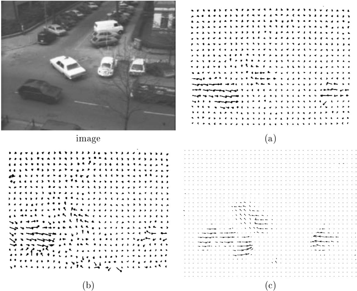
FIGURE 7. **Hamburg Taxi Sequence, other algorithms.** The flow field results by Anandan’s algorithm are shown in (a). The flow field by Singh is shown in (b). Both of these diagrams appear in Barron et al. [5]. Our results were resampled and are shown in a similar format in (c).
