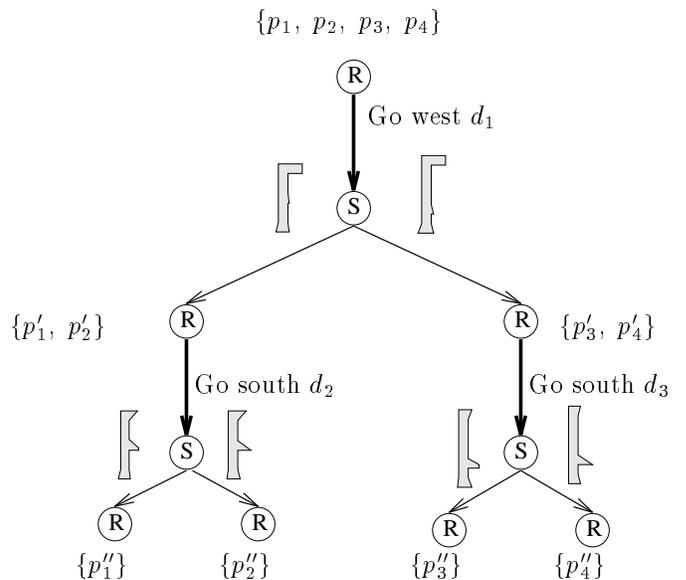
Figure 2: A map polygon and 4 hypothetical locations  $\{p_1, p_2, p_3, p_4\}$  with a localizing decision tree for determining the true initial position of the robot.
