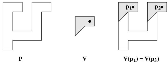
Figure 1: Given a map polygon  $P$  (left) and a visibility polygon  $V$  (center), the robot must determine which of the 2 possible initial locations  $p_1$  and  $p_2$  (right) is its actual location in  $P$ .
