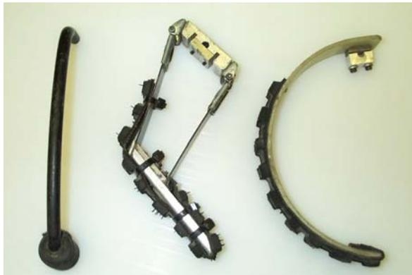
Figure 9 - Evolution of legs for Research-RHex, half-circle leg on right
