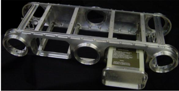
**Figure 4 - Rugged-RHex frame - shown with battery in carrier**
