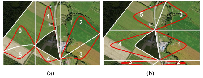
Fig. 3. Results of off-line analysis using (a) the default direction of coverage, and (b) after aligning with the dominant axis of the free space.
