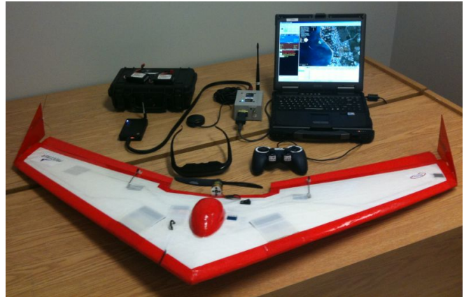
Fig. 1. Our robotic platform is a commercial fixed-wing UAV with an on-board autopilot microprocessor and a gimbal-mounted camera.
