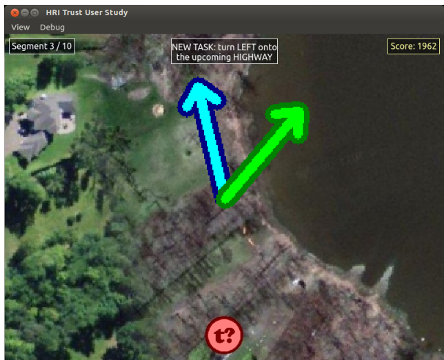
Figure 1: Live camera feed from an aerial robot overlaid with an autonomous boundary tracker’s steering command (blue arrow), and the human’s interventions (green arrow). Additional overlays are pertinent to our observational study (see Sec. 3).
