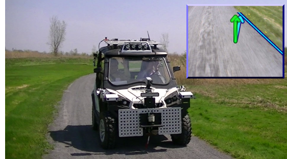
Figure 1: Our interactive, adaptive vehicle tracking a road. Inset: camera view overlaid with tracked boundary (blue line), robot’s steering (blue arrow), and human’s intervening command (green arrow).
