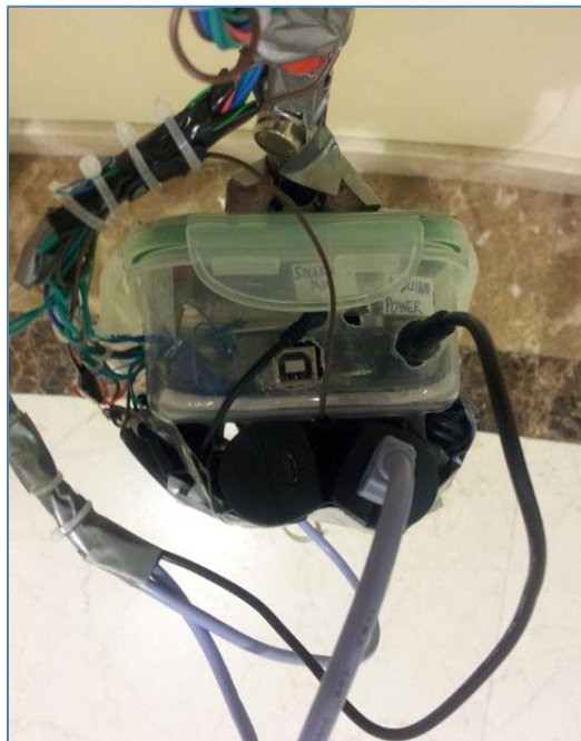
Figure 83: Close View of Holes Made into the Microcontroller and Circuit Box for Different Cables
