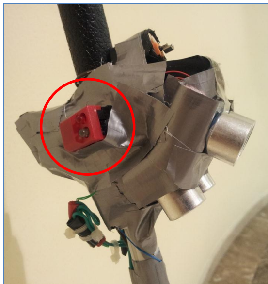
Figure 73: Closer View of Emergency Trigger Switch
