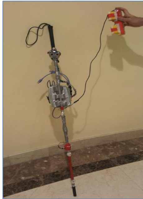
Figure 80: View of the Kinetic Generator Ready for Shaking and Charging the Batteries
