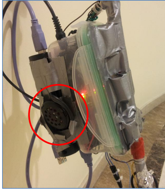
Figure 74: Closer View of the Speaker for Locating the Stick
