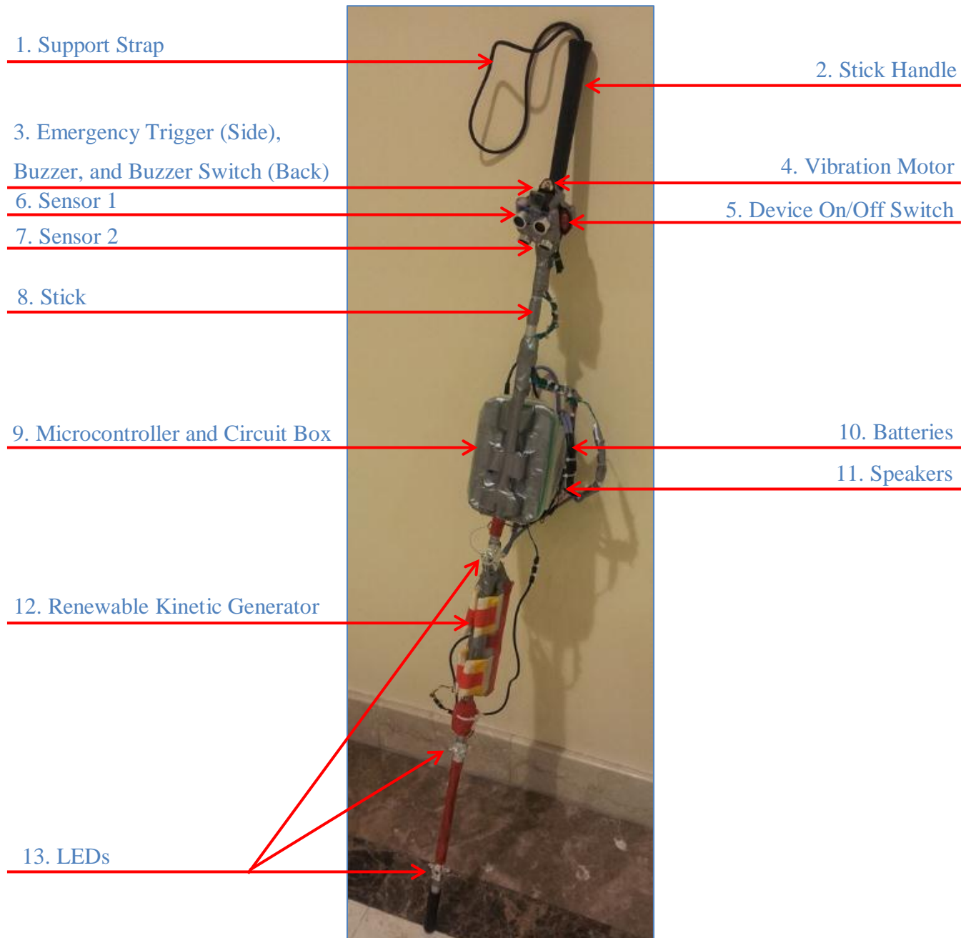
Figure 72: Final Prototype of the Self-Energized Smart Vision Stick
