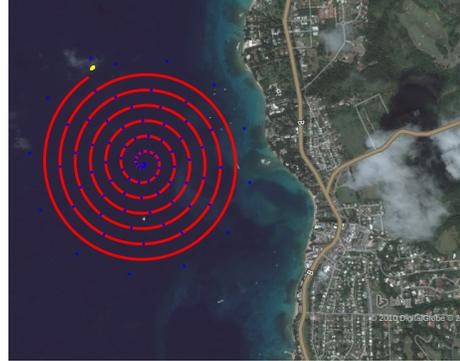
Fig. 1: Simulated spiral search pattern on Microsoft Bing Maps ©. The red dots indicate the waypoints of an ASV and the yellow dots represent the drifter waypoints.
