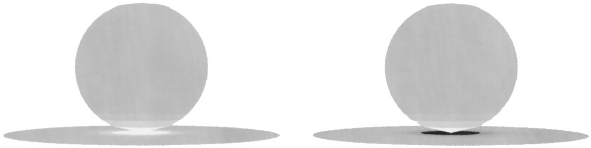
Figure 2. Two interreflection modes \mathbf{I}_0 and \mathbf{I}_1 for a sphere resting on a disk. (Black indicates negative values, white indicates positive, and grey indicates zero.) The mode on the left has the largest eigenvalue of all modes ( \mu_0 = 0.83 ) and the mode on the right has the smallest eigenvalue ( \mu_1 = -0.83 ). The functions \mathbf{I}_0 and \mathbf{I}_1 are identical in absolute value. \mathbf{I}_0 is positive everywhere, and \mathbf{I}_1 is positive on the sphere but negative on the disk. The next few interreflection modes (not shown) have similar eigenvalues. These modes differ from the first two by having a sinusoidal variation (of period 2\pi radians) as a function of longitude angle.
